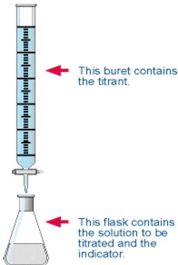
**Setup for a Typical Titration** In a typical titration, the titrant in the buret is added to the solution in the Erlenmeyer flask until the indicator changes color to show that the reaction is complete.
