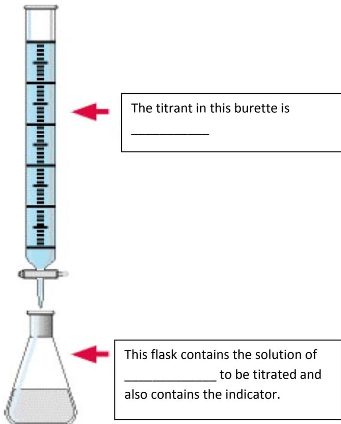
The indicator that we will use in this lab is phenolphthalein. It will turn pink when the HCl solution in the flask becomes the slightest bit basic. The HCl will become basic because we're adding NaOH slowly from the burette.
